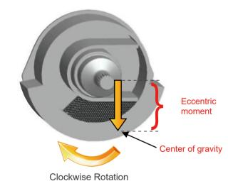
■ The position of the steel shot and the eccentric weight combine to produce the maximum centrifugal force
